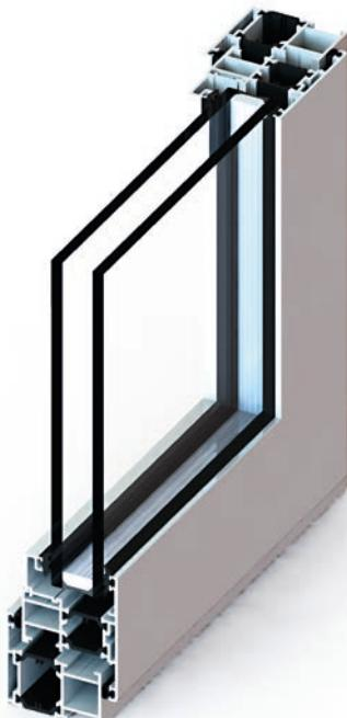
Technically advanced framing systems with slim sight lines. The KWS Window Suite is fabricated using a mechanical corner cleat, which ensures easy and fast fabrication times. KWS is available in both 51 mm and a 75 mm wide profile sections.
